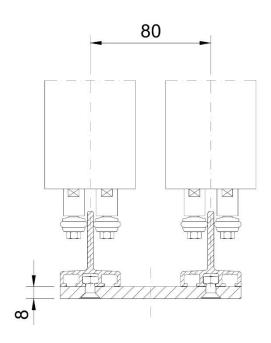
As the shutter height is determined by the clear height, and the fin center to center distance is fixed per fin type, a distance "X" remains. This distance will equally be divided at the top and bottom of the shutter.
