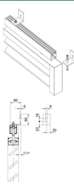
Loads, applied on the rails brackets come from the dead weight of the shutters and wind induced pressure and suction on the shutters :
